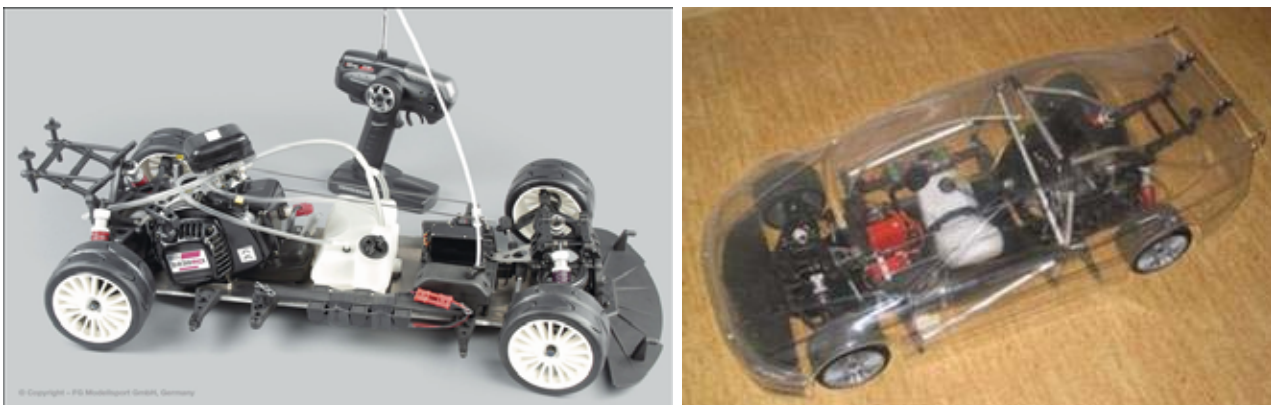
Fig. 1. Model of vehicle (in scale 1:5) –vehicle building kit of firm FG Modellsport [1]
